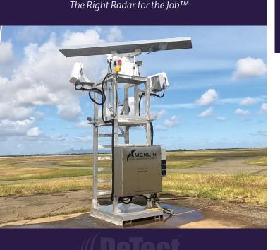
Proven bird radar technology tested, validated & used operationally by commercial airports, the US Fish & Wildlife Service, Air Force, Navy & NASA
