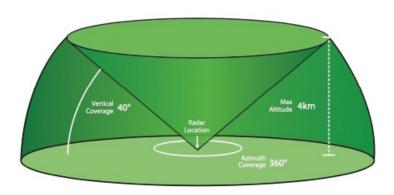
Unlike traditional 3D & quasi-3D radars that scan only one sector at a time and leads to under-sampling, fewer tracks & low accuracy altitude estimates, DeTect's dynamic multibeam True3D radar scans & updates target data across the entire 3D volume continually, providing precise (x-y-z) data and no target or track error.
