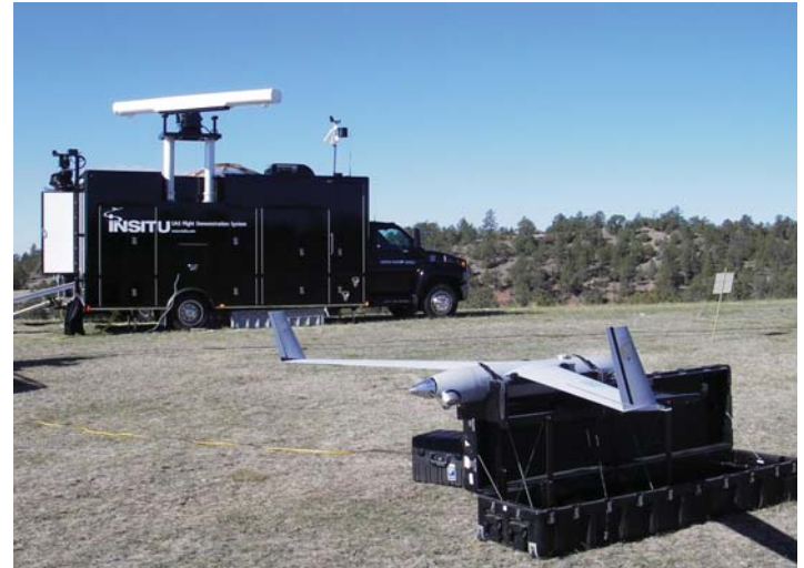
ABOVE: HARRIER GBSAA system installed into customer-provided UAV operations support vehicle.
