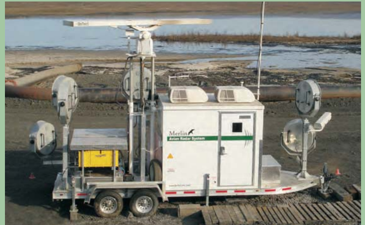
ABOVE: MERLIN detect & deter system installation at oil sands processing facility waste pond in northern Canada providing migratory bird control; networked system includes three self contained master radar trailers & over ten satellite deterrent unit trailers.
