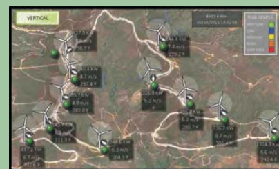
(Right) MERLIN SCADA-R interface for raptor mitigation using turbine centric model that idles individual turbines when proximate risk is detected; each turbine is assigned a color-coded risk value (El Pino wind farm, Spain)
