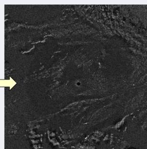
(Above right) - Horizontal radar image from a solid state, X-band radar, and Doppler filters applied to filter out stationary (zero velocity) targets.
