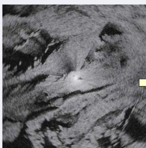
(Above left) - Initial horizontal radar image from a magnetron S-band radar. Light areas represent extensive ground clutter produced by vegetation with high water content abundant at the test site; target detection and tracking was poor or impossible in these areas.
