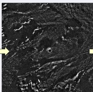
(Above middle) - Horizontal radar image produced by a 5.5-m solid state, X-band radar with a Doppler processor. No Doppler filters were applied to this image, and white areas still show some areas with high ground clutter.
