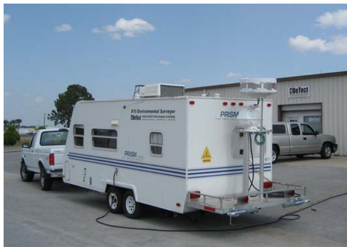
Figure 4: Prototype MERLIN Fixed-beam Vertical Profiler Radar currently in field testing.
