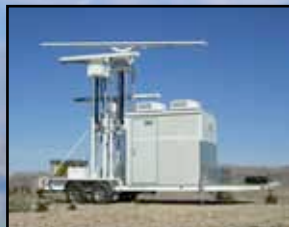
Figure 2. MERLIN XX25200e Avian Radar System with enhanced resolution.
