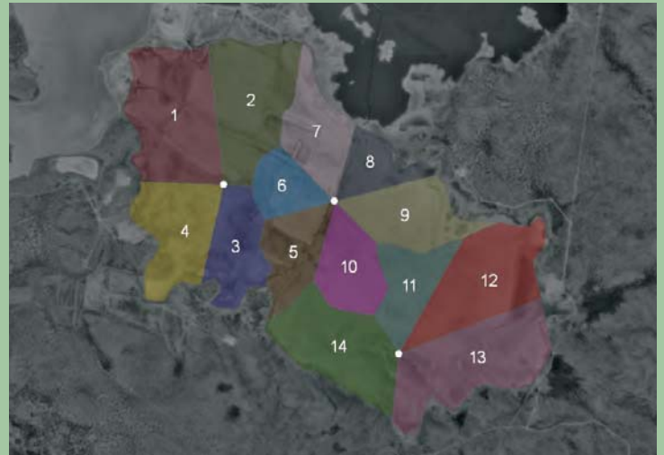
BELOW: MERLIN detect & deter hazing activation zones (14 total) for product evaporation ponds at potash mine in the southwestern U.S.; networked three trailer system.
