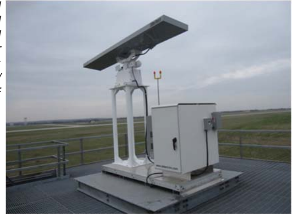
Right: Fixed Mounted Horizontal Sensor Platform; GBSAA / HSR-F
