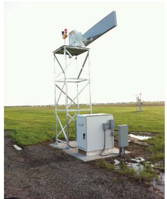
Right: Fixed Mounted Vertical Sensor Platform; GBSAA / VSR-F
