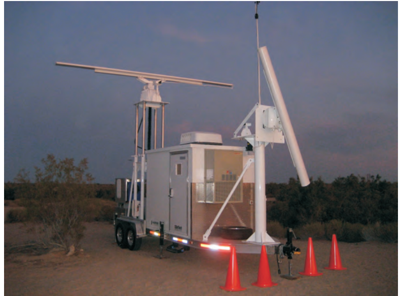
Upper photo: Mobile HARRIER BSR dual ground-air surveillance radar system installation in western US desert; includes radar directed slew-to-track long range day-night camera unit.
