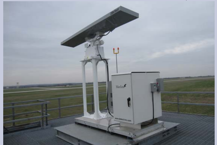
BELOW: MERLIN systems are also available in fixed, fully self-contained skid package units (MERLIN SS200d HSR sensor installation at US Air Force Whiteman AFB, Missouri USA.)
