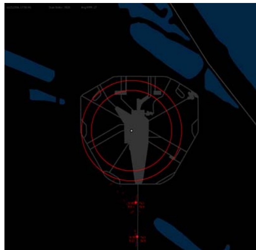
Custom NASA MERLIN HSR display with space shuttle nosecone centered in screen and risk zones defined; from NASA MERLIN ARS, Kennedy Space Center, Florida, USA
